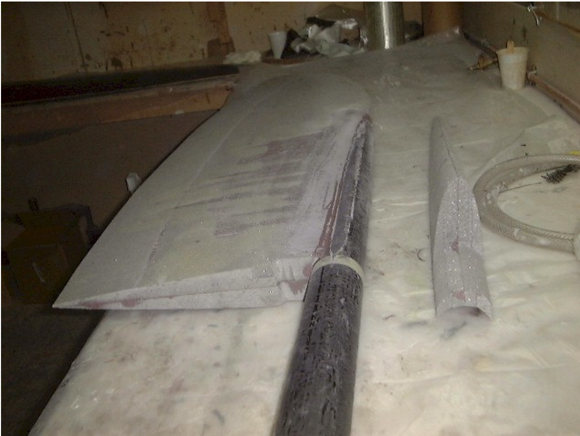
On this C&C110 rudder, the post is being fitted to the core. Uni carbon will wrap around the core and post prior to bonding on the leading edge of the core (sitting to the right in this photo).
