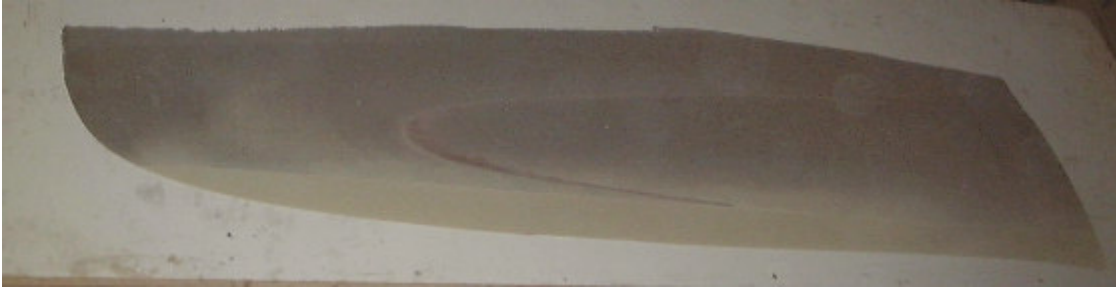
This Aerodyne 38 core was machined with a strip of high density foam along the leading edge.
