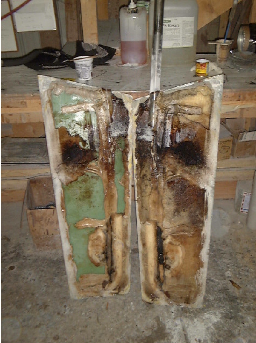
Sirius 28 rudder after splitting apart.
