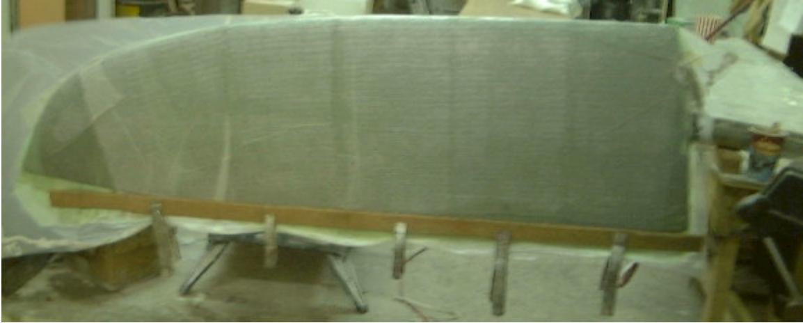
C&C37R rudder in the vacuum bag. Battens are clamped along trailing edge to eliminate distortion.
