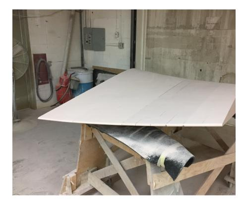
As Philip explains, here at CCI we were challenged with the construction of the tooling for a unique highly-bent and twisted wind blade that is about 40' from tip to tip when measured along its surface. We'll be making three of these blades, which together form Biome's PowerCone® technology.
